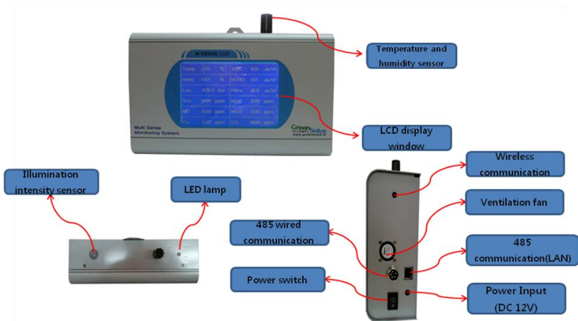
<Figure 3> Real-time monitoring system device for preservation environment
